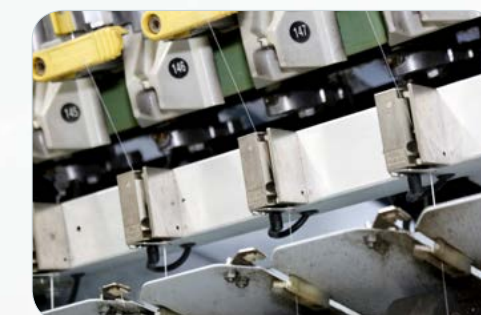
【在线张力检测装置】 On-line yarn tension detecting device
