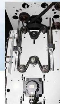
伺服成型 Traverse by servo drive
