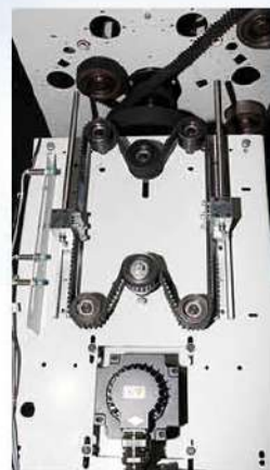
伺服成型 Traverse by servo drive
