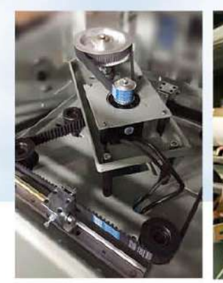
伺服成型 Traverse by servo drive
